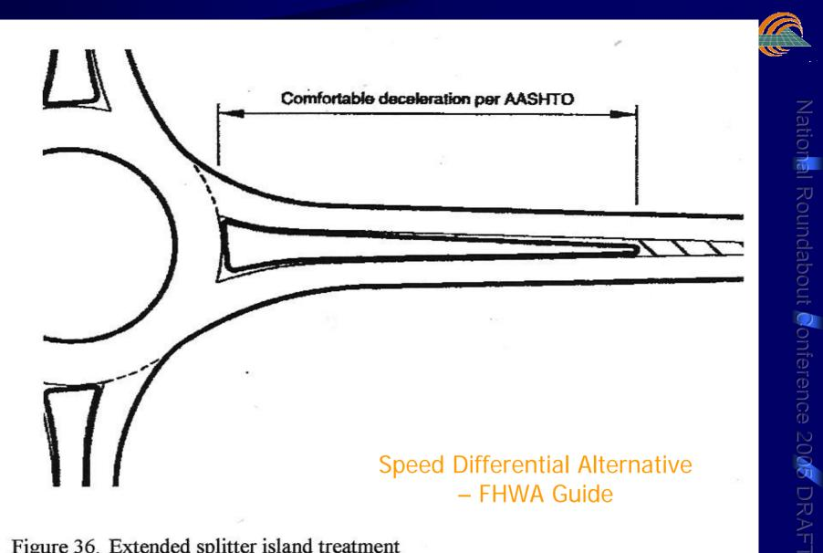
Figure 36. Extended splitter island treatment
