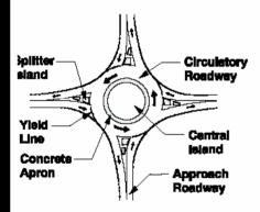
Roundabouts are designed to accommodate fire trucks and large vehicles. Large trucks may have to drive on the concrete island around the central island in order to get through the roundabout.
