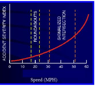
Figure 3: Accident Severity & Speeds (Courtesy: Mark Johnson)
