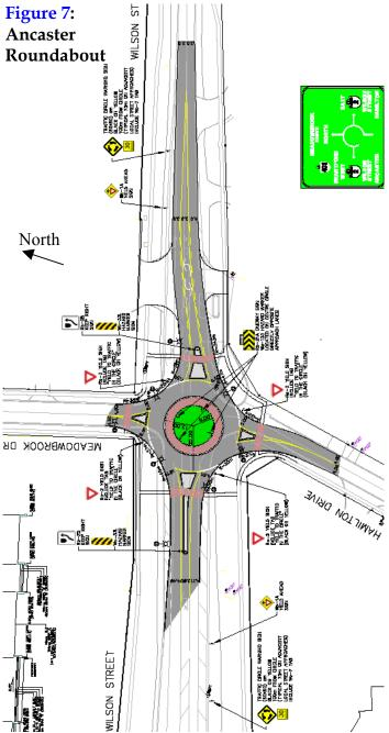
opened in 2002. The dates of the roundabout data are shown in the table. **Figure** 7 above illustrates the implemented design for the Ancaster Roundabout.
