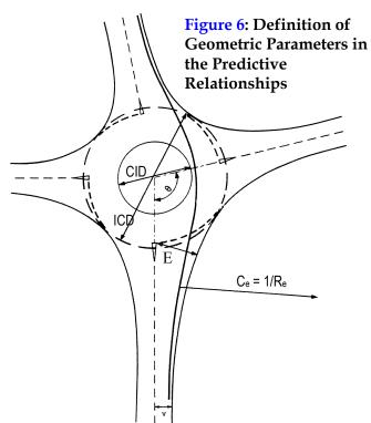
relationships are shown in **Figure 6**. The costly research undertaken in the early 1980's using four years of data has identified relationships between safety and geometry for a wide range of traffic flows and geometric conditions.
