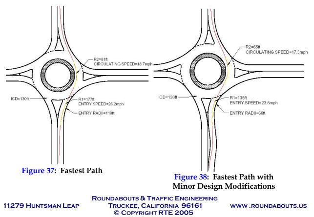
There are two alternative design treatments for splitter island design aimed at mitigating the effects of high rates of speed of traffic approaching a roundabout.
