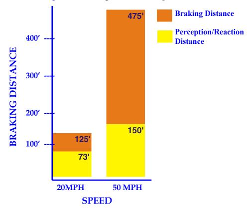
Figure 2: Braking Distances & Speeds
