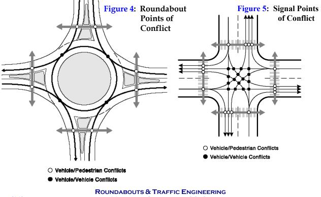
TRUCKEE, CALIFORNIA 96161 © COPYRIGHT RTE 2005 As shown above, there are 32 points of conflict at a signalized intersection with only 12 points of vehicular and pedestrian conflicts at a roundabout. This solves the question in a very basic way of why roundabouts are safer than a signalized intersection.
