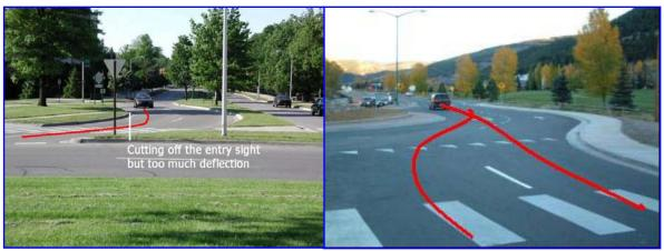
**Figure 35:** An Over-deflected Entry (But good use of landscaping on the splitter island prior to entry) **Figure 36:** Insufficient Entry Path Curvature (*This layout also suffers from an entry path overlap creating safety and capacity issues*)
