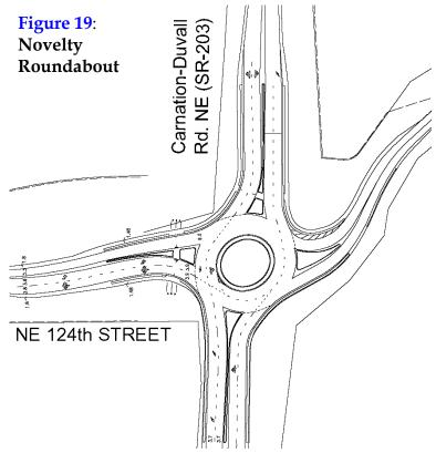
roundabout design plan conceptual layout and **Figure 20** for a vicinity map of the Washington area where the Novelty Roundabout is located.
