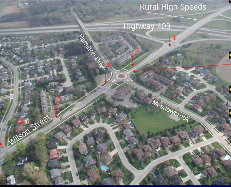
🙆 Design Works With Rural High Speed Approach Elongated Splitter Island Adequate Deflection 6 Point Speed 20 ğ Corridor Study Conducted
