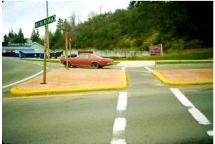
Figure 11 - Cross Walk Alignment That Is Too Enticing
