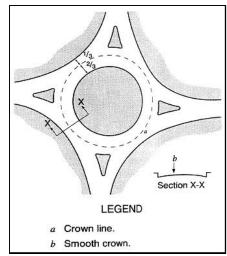
Figure 15 - Setting the Crossfall For Multi-Lane Roundabouts (10)
