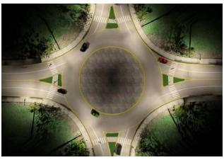
Figure 14 - Approach Mounted Lighting 8-250W HPS (Courtesy: DMD Associates Electrical Consultants)
