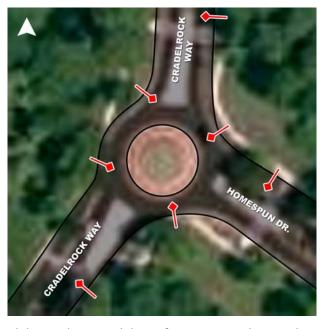
• For vehicles approaching the roundabout, the roundabout features are clear and conspicuous. Drivers have the ability to see and react to other vehicles approaching or circulating in the roundabout.
