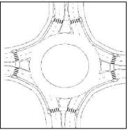
Roundabouts have raised splitter islands at each approach that separate the entry and exit lanes of a street. These splitter islands are designed to deflect traffic and thus reduce vehicle speed. Splitter islands also provide a pedestrian refuge between the inbound and outbound traffic lanes.
