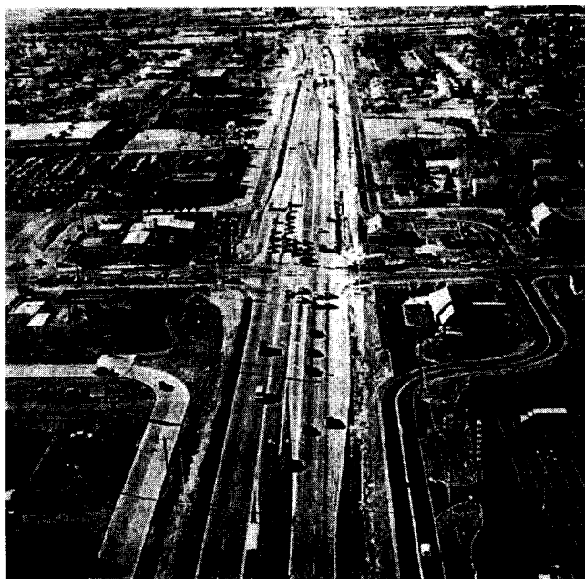
Figure 8-7. Divided arterial streets with 2-way frontage road.
