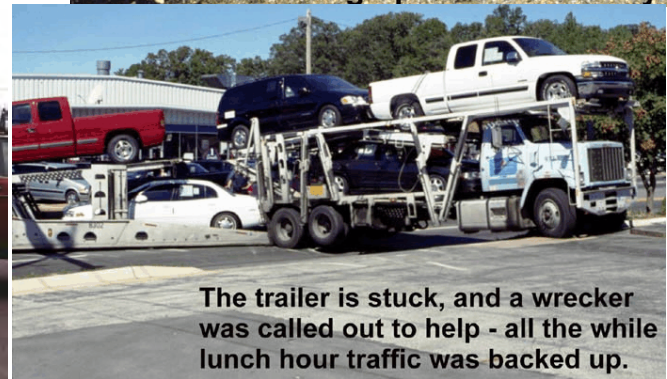
EXHIBIT 3-40 Driveway grade and roadway cross slope problems
