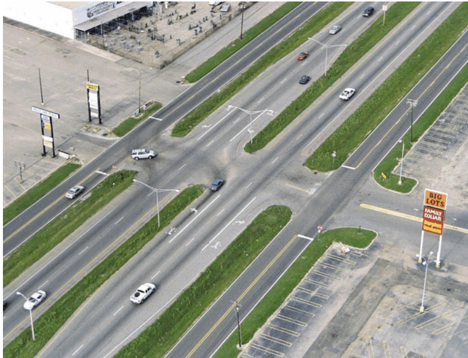
EXHIBIT 3-33 Frontage road intersection with cross street too close
