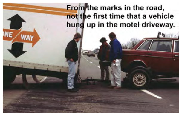
EXHIBIT 3-40 Driveway grade and roadway cross slope problems
