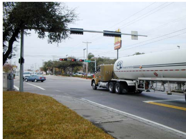
Truck unable to complete turn within short signal timing. If truck stops in current position, trucks turning right will be unable to negotiate the turn without running over the sidewalk.
