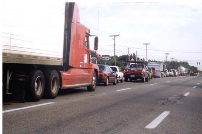
Signal timing can cause vehicles to back up into through lanes if turn lanes are not long enough to accommodate the queue.
