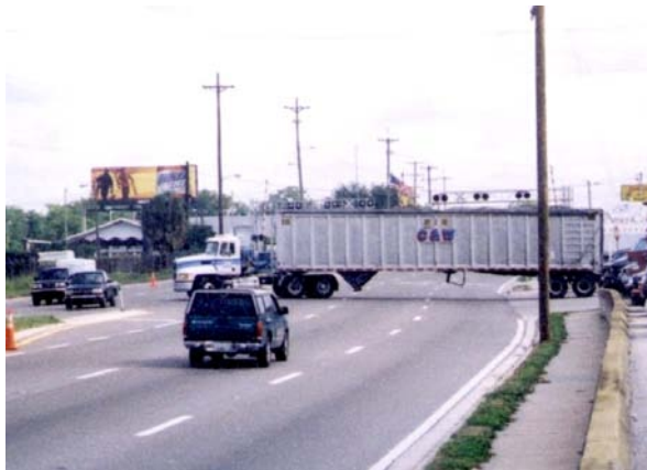
Truck blocks three lanes of traffic waiting for gap in opposing lanes to complete left turn through median.
