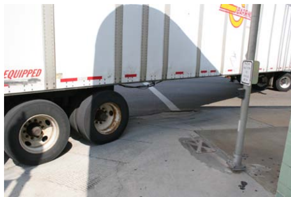
Truck maneuvers around tight corner tracking over curb and narrowly missing overhang of nearby structure located at the intersection of US 301 and SR 54.
