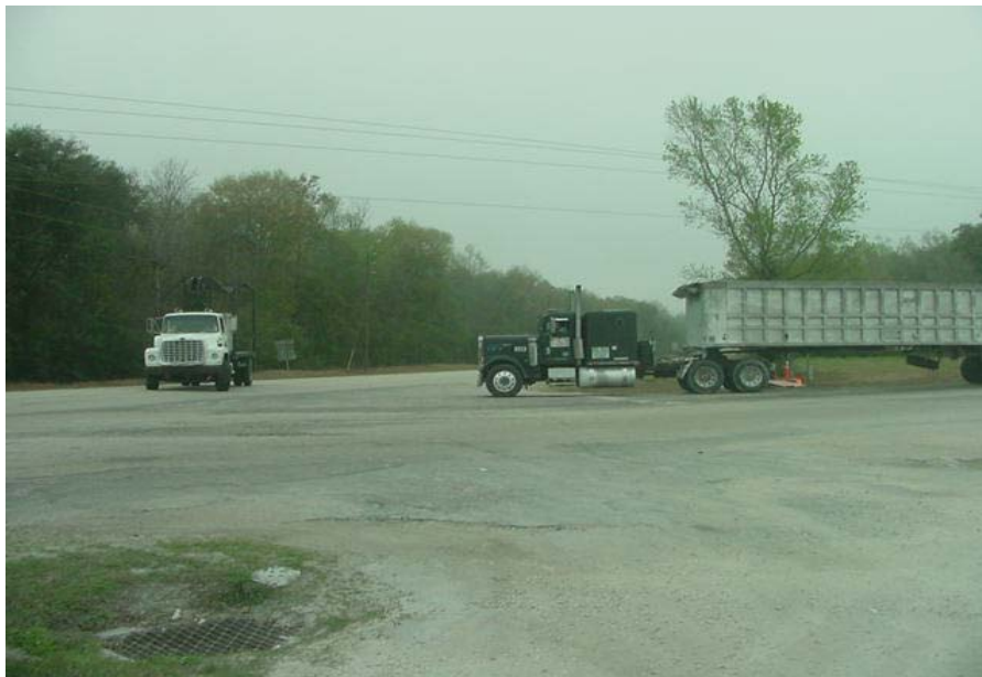
At skewed intersections that experience heavy truck traffic, truckers have difficulty seeing traffic traveling at high speeds.
