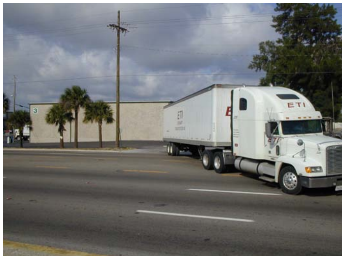
Truck exits driveway blocking southbound lanes while attempting a left turn through median.
