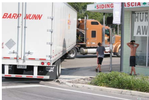
Truck tracks over sidewalk while making wide turn into on-coming traffic. Note the building overhand that extends over the sidewalk almost to the curb which adds to the difficulty of this turn for trucks.
