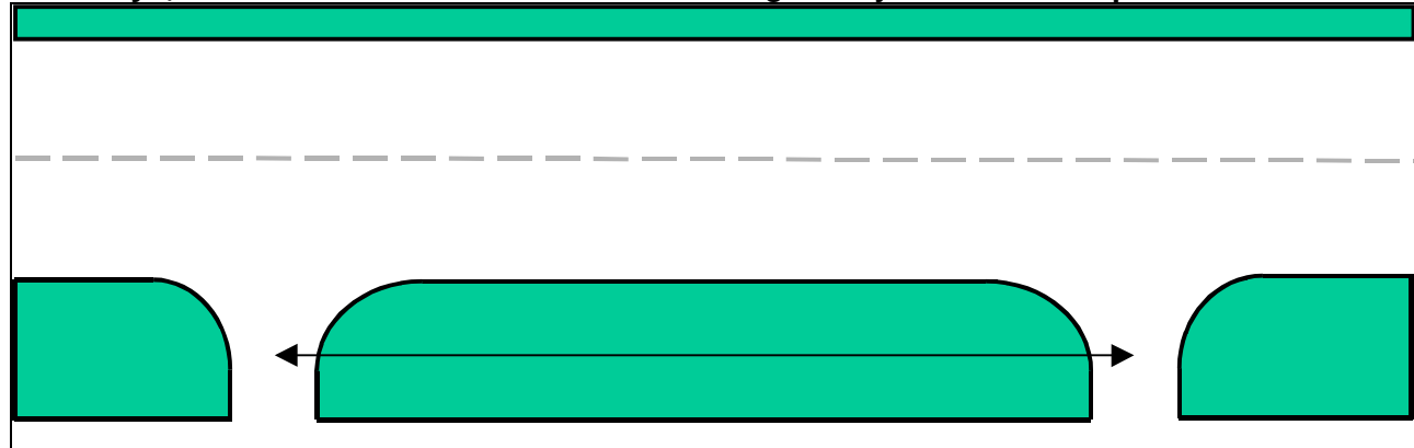
Figure 20—Driveway spacing guidelines: Adopt minimum spacing requirements for driveways, and reinforce with minimum lot frontage and joint access requirements
