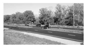
*Figure 15. Conventional median opening at three-leg intersection.*
