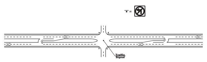
b) Signalized Four-Leg Intersection With No Turns Permitted and Two Directional Midblock Median Openings
