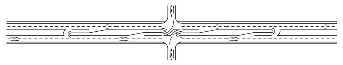
b) Directional Median Opening Four-Leg Intersection With Two Directional Midblock Median Openings (Type 2b + Type 6a + Type 2b) *Figure 48. Conventional and directional median openings at four-leg intersection.*
