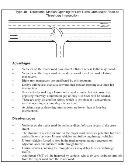
*Figure 30.* Advantages and disadvantages of median opening type 4b directional median opening for left turns onto major road at three-leg intersection.
