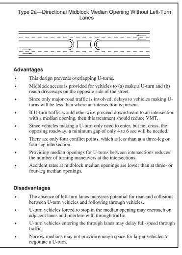
*Figure C-6.* Advantages and disadvantages of median opening type 2a—directional midblock median opening without left-turn lanes.
