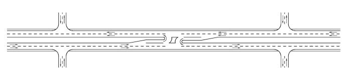
*Figure 41.* Combination C4—directional midblock median opening between four-leg intersections without median openings.
