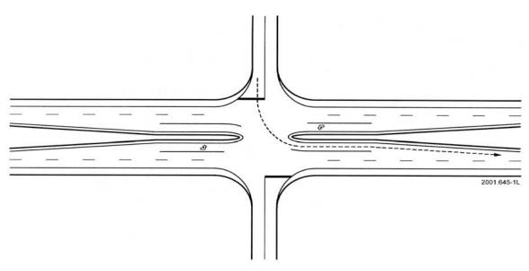
Figure 6. Typical divided highway intersection with median acceleration lanes (7).
