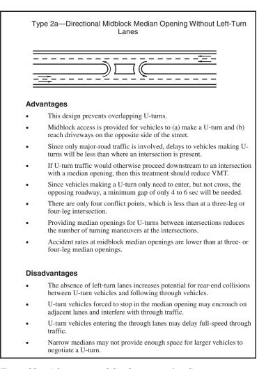
*Figure 22.* Advantages and disadvantages of median opening type 2a—directional midblock median opening without left-turn lanes.
