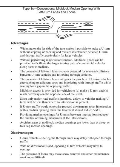
*Figure 21.* Advantages and disadvantages of median opening type *lc*—conventional midblock median opening with left-turn lanes and loons.
