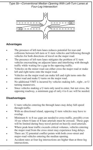
*Figure 32.* Advantages and disadvantages of median opening type 5b—conventional median opening with left-turn lanes at four-leg intersection.
