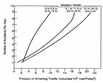
Figure 4. Variation of annual accident frequency at divided highway intersections as a function of median width and exposure index (the product of the ADTs of the intersecting roadways) (10).
