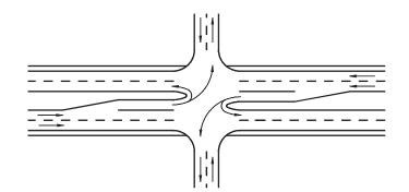
a) Conventional Median Opening at Four-Leg Intersection (Type 5b)
