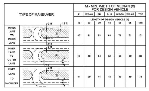
Figure C-18. AASHTO minimum median widths to accommodate U-turns (3).
