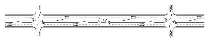
*Figure 40. Combination C3—Directional midblock median opening between four-leg intersections with conventional median openings.*
