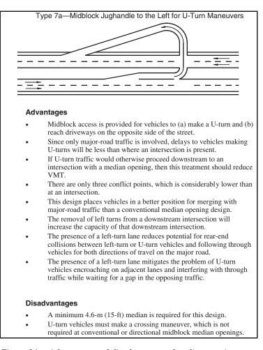
*Figure 34.* Advantages and disadvantages of median opening type 7*a*—midblock jughandle to the left for U-turn maneuvers.
