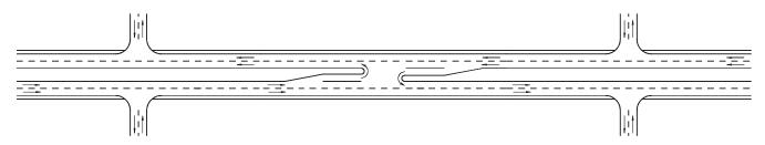
*Figure 43.* Combination C6—conventional midblock median opening between four-leg intersections without median openings.
