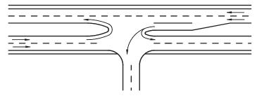
a) Conventional Median Opening at Three-Leg Intersection (Type 3b)
