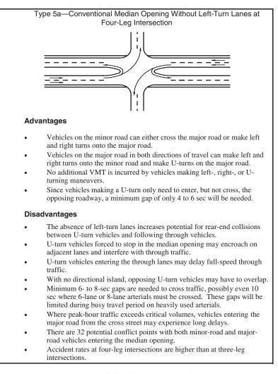
*Figure 31.* Advantages and disadvantages of median opening Type 5a—conventional median opening without left-turn lanes at four-leg intersection.
