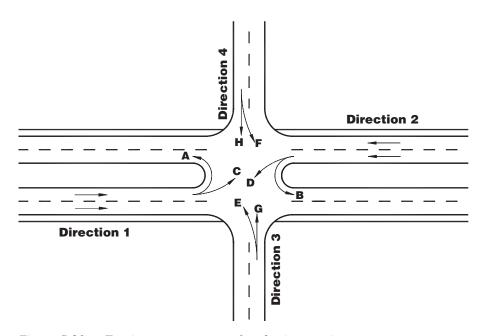
Figure C-20. Turning movements at a four-leg intersection.
