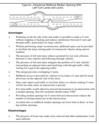
*Figure C-8. Advantages and disadvantages of median opening Type* 2*c*—*directional midblock median opening with left-turn lanes and loons.*
