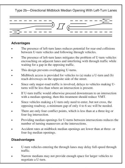
*Figure 23.* Advantages and disadvantages of median opening type 2b—directional midblock median opening with left-turn lanes.
