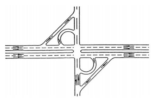
*Figure 9.* At-grade loop (surface loop) with crossroad (3).
