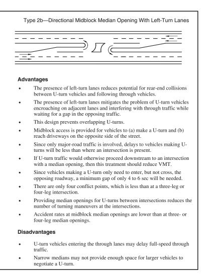
*Figure C-7.* Advantages and disadvantages of median opening type 2b—directional midblock median opening with left-turn lanes.
