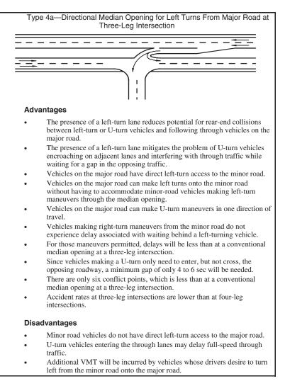
*Figure 29.* Advantages and disadvantages of median opening type 4a—directional median opening for left turns from major road at three-leg intersection.
