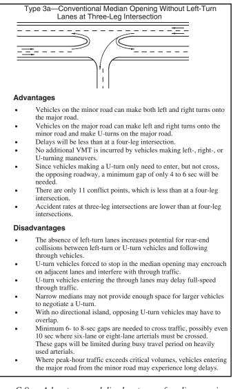
*Figure C-9.* Advantages and disadvantages of median opening type 3a—conventional median opening without left-turn lanes at three-leg intersection.
