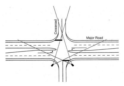
Figure 46. Typical data collection setup using video cameras (8).
