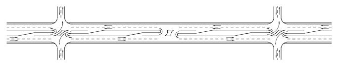
*Figure 38.* Combination C1—directional midblock median opening between four-leg intersections with directional median openings.
