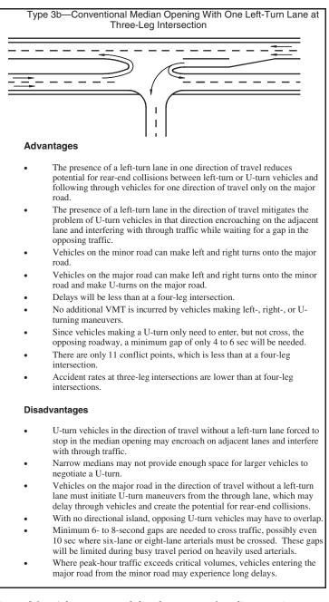
*Figure 26.* Advantages and disadvantages of median opening type 3b—conventional median opening with one left-turn lane at three-leg intersection.
