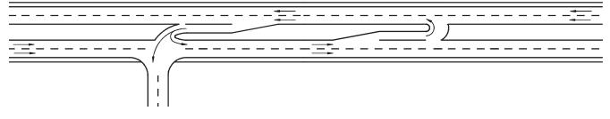
b) Directional Median Opening For Left Turns From Major Road at Three-Leg Intersection With Directional Midblock Median Opening (Type 4a + Type 2b)
