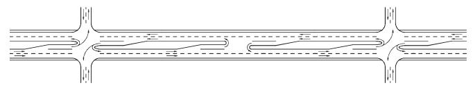
*Figure 39.* Combination C2—Conventional midblock median opening between four-leg intersections with conventional median openings.
