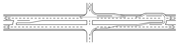
Figure 7. Typical loon design at a directional median opening (55, 56).
