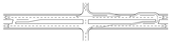
Figure C-19. Typical loon design at a directional median opening (55, 56).
