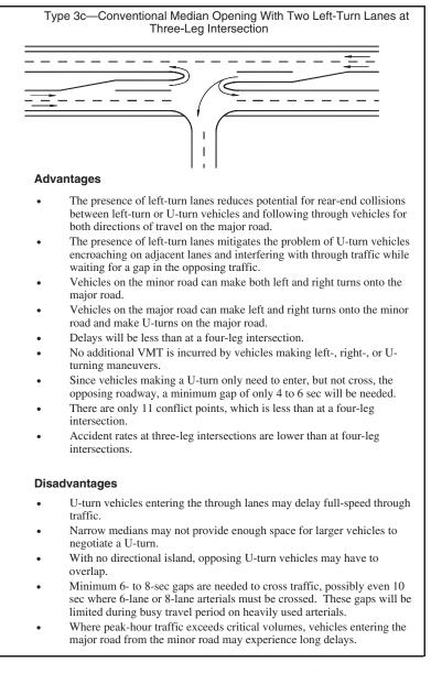
*Figure C-11.* Advantages and disadvantages of median opening type 3*c*—conventional median opening with two left-turn lanes at three-leg intersection.
