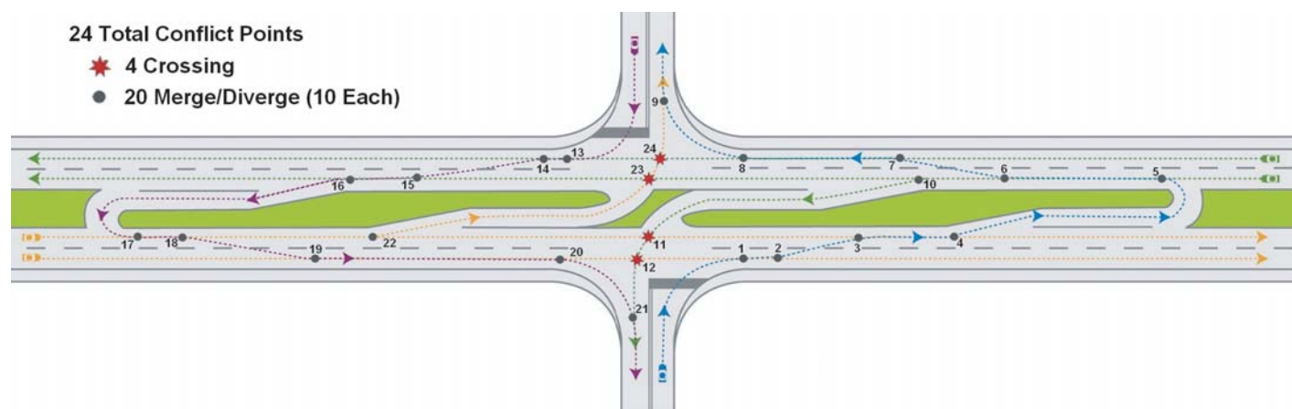
Figure 48. Conflict-point diagram for J-turn intersection.
