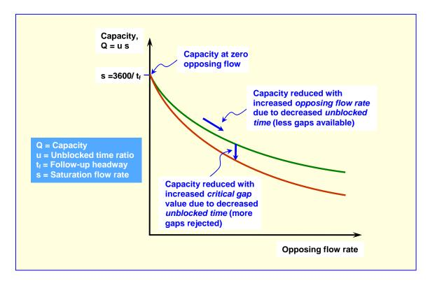
Figure 1 - Gap-acceptance capacity
