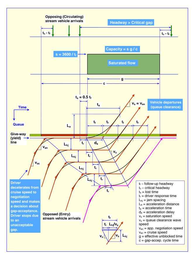
Figure 3 - Gap-acceptance capacity and queue discharge parameters
