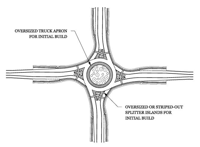
FIGURE 2 Example of initial outside build with future inward widening.
