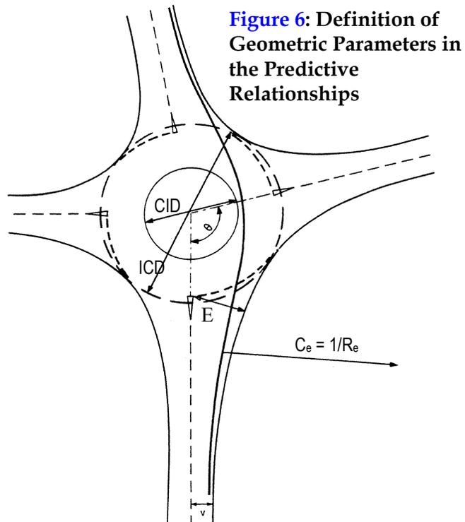
**Figure 6: Definition of Geometric Parameters in the Predictive Relationships**
