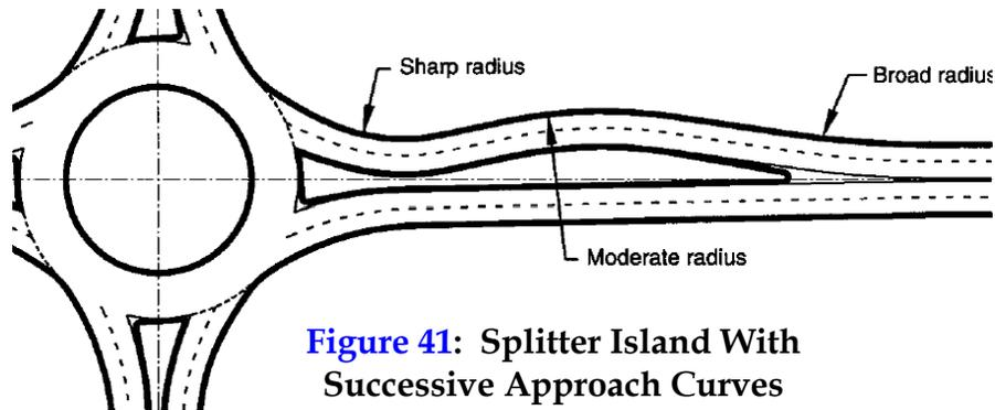
**Figure 41: Splitter Island With Successive Approach Curves**
