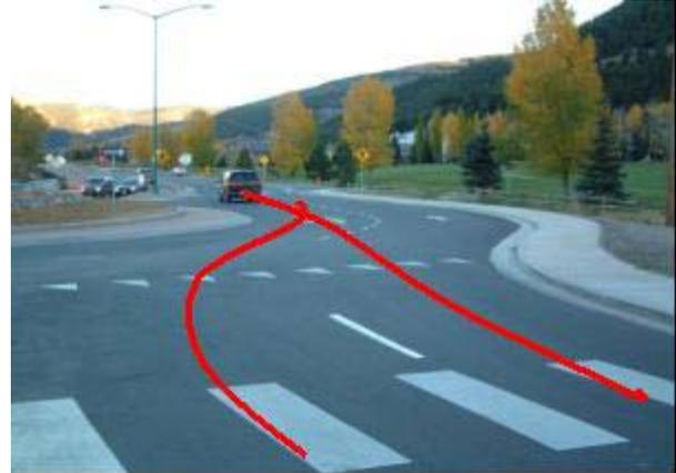
Figure 3 - Insufficient Entry Path Curvature
