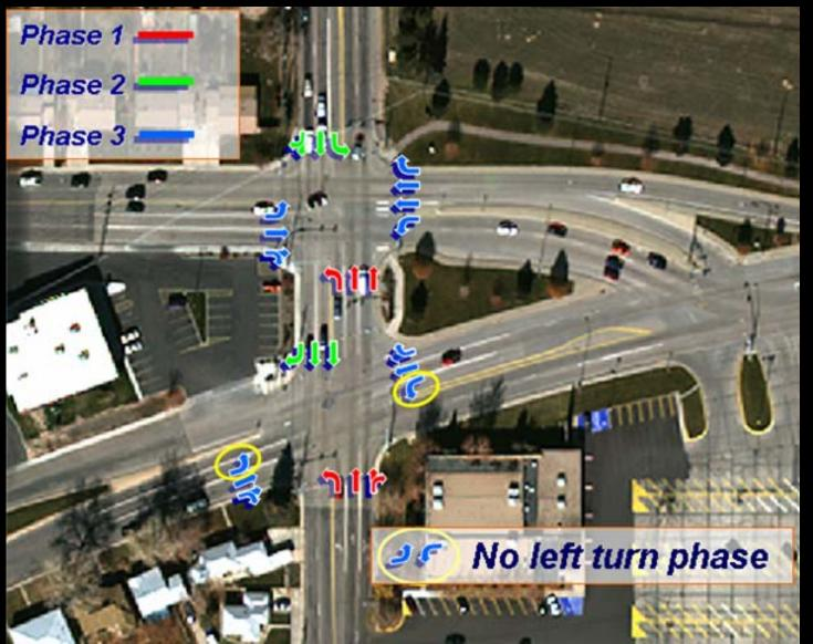
> Split phase signal timing impacts intersection capacity
